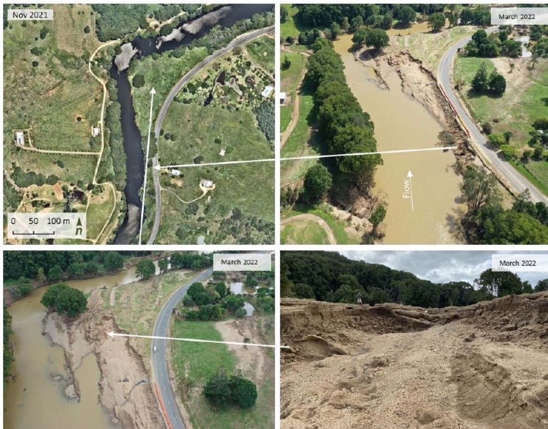
Figure 3.4 Damage examples from Flood 2022. Formation of a chute channel across the floodplain and significant bank retreat up to edge of Kyogle Road. (Source: Alluvium, 2022)
