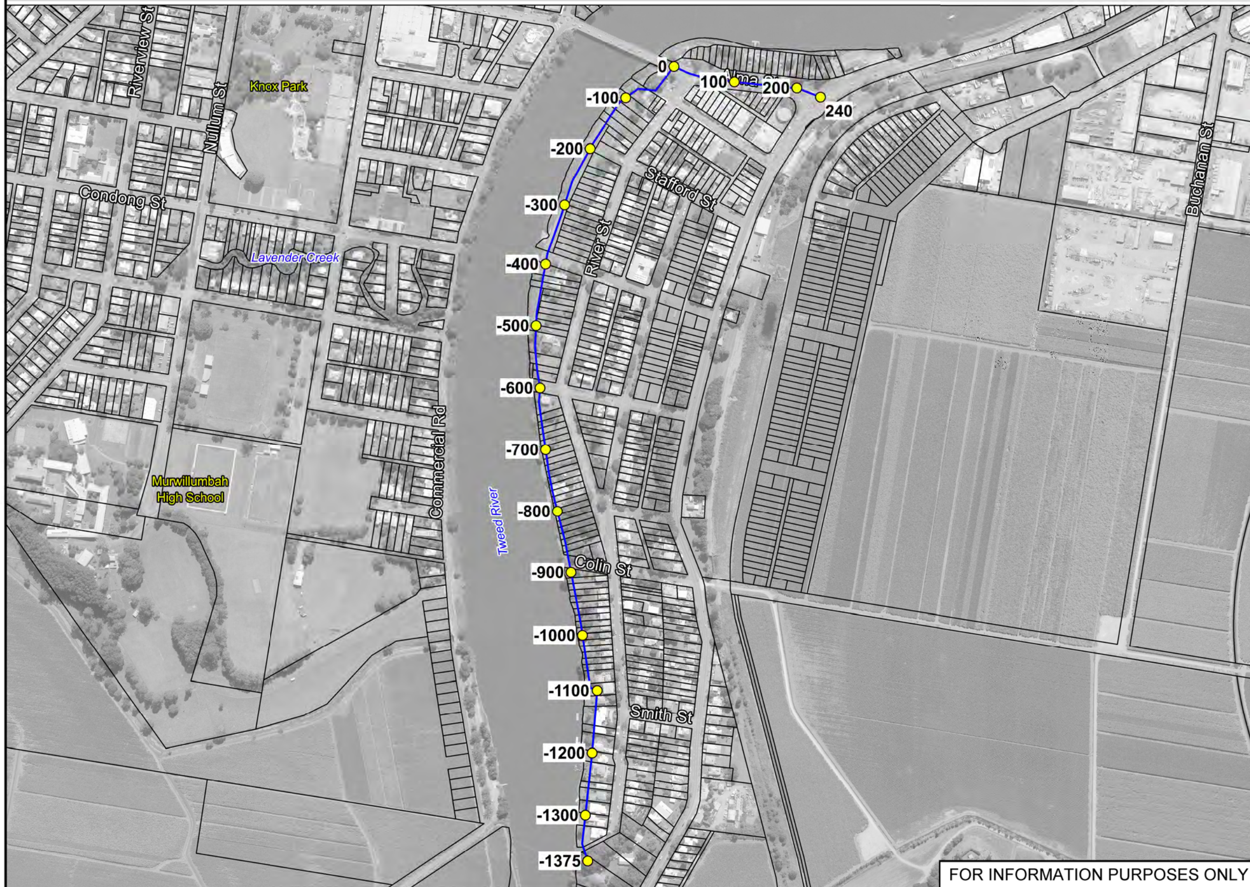
Figure 41.2: Concept Design for Raising the South Murwillumbah Levee to 5% AEP and Raising Height of the CBD Levee (FM9)
