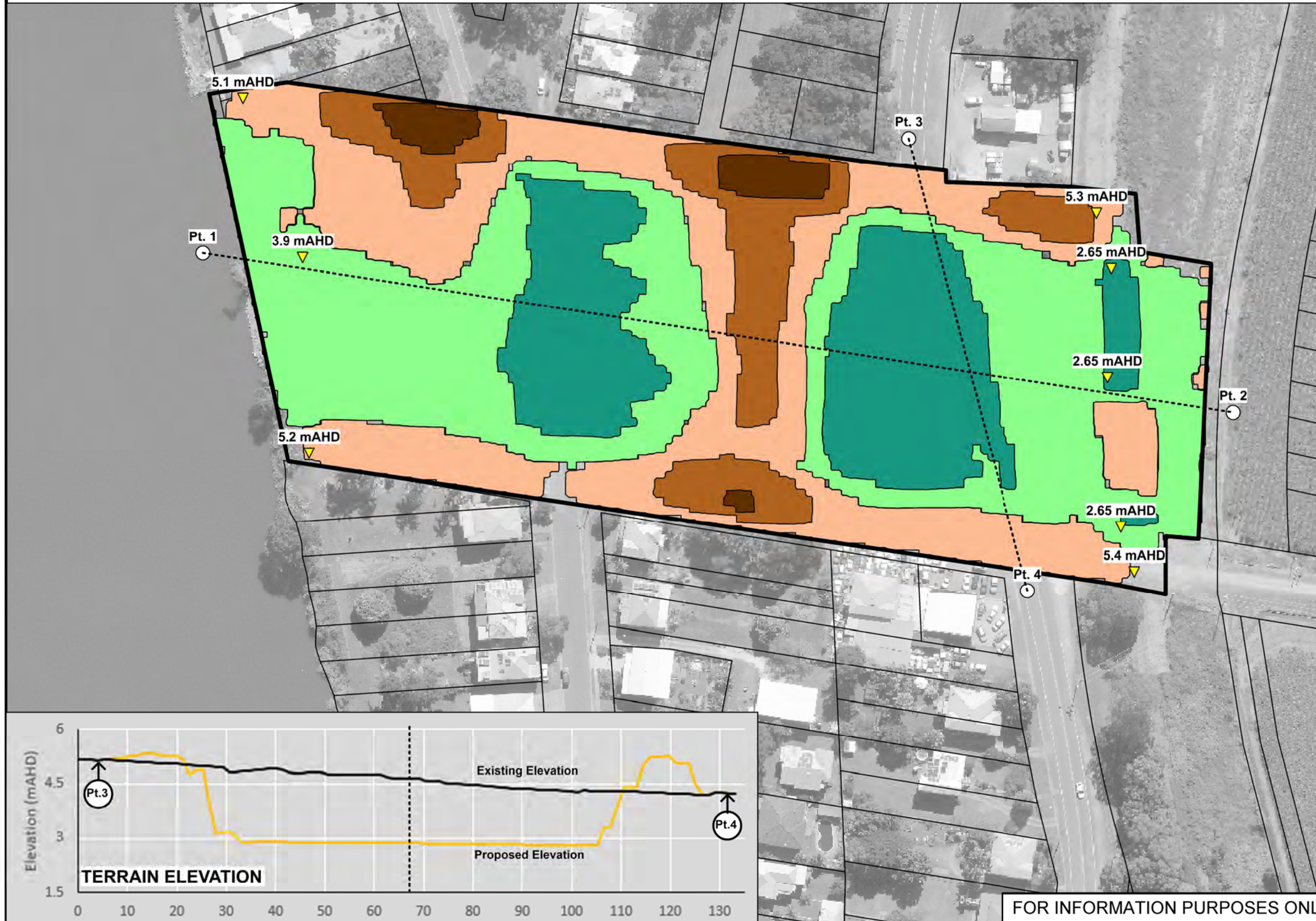
Figure 34.2: Concept Design for the South Murwillumbah High Flow Bypass Option 1 (FM2)
