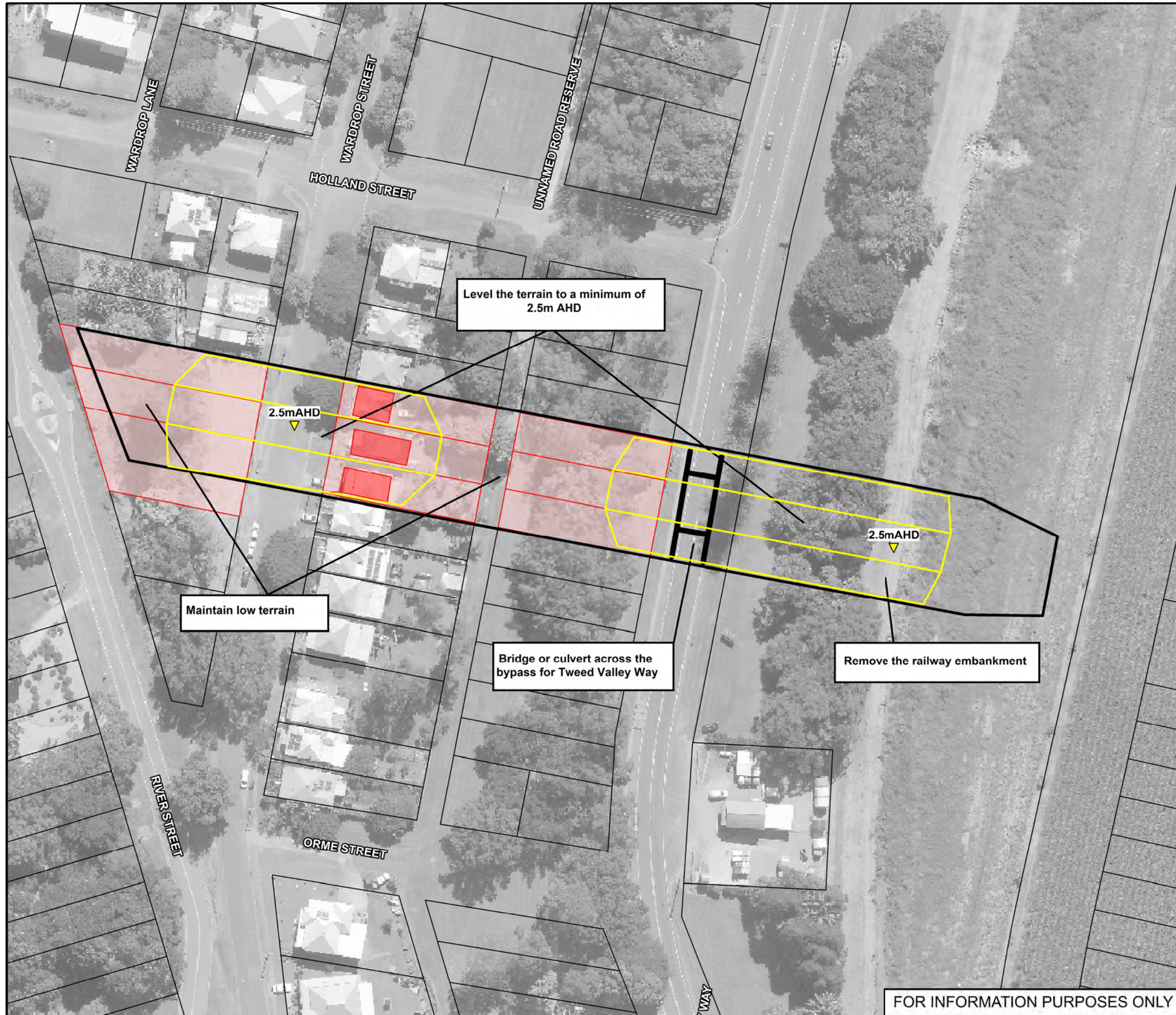
Figure 35.1: Concept Design for the South Murwillumbah High Flow Bypass Option 2 (FM3)
