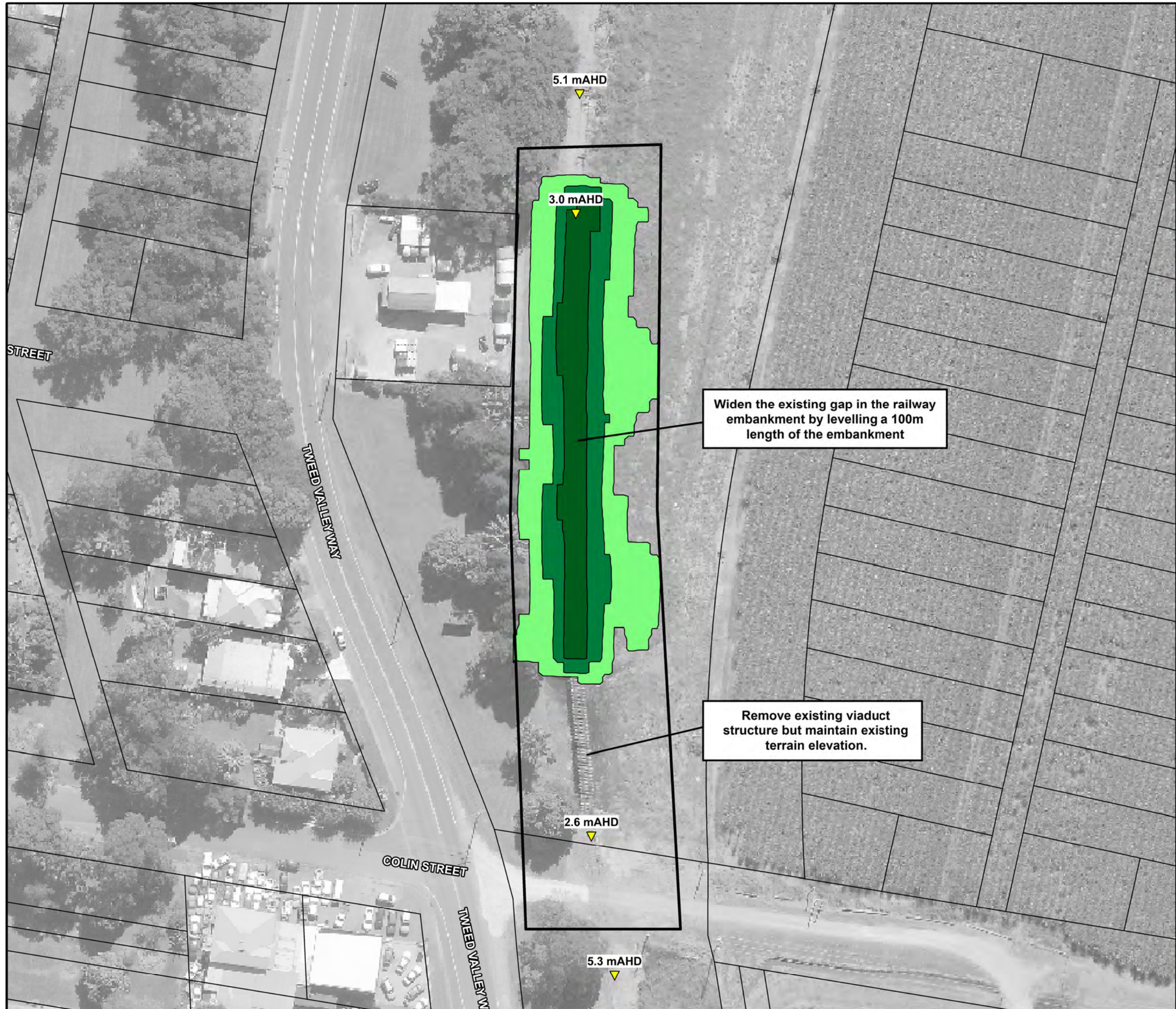
Figure 43: Concept Design to Modify the Railway Embankment (FM11)
