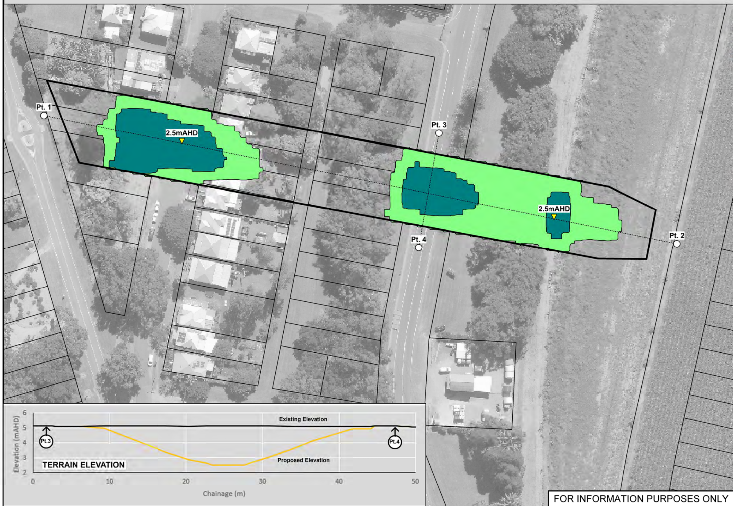
Figure 35.2: Concept Design for the South Murwillumbah High Flow Bypass Option 2 (FM3)
