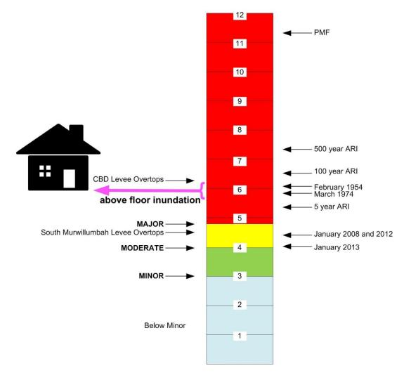
Figure 4–1 Floor Level to Gauge Relationship
