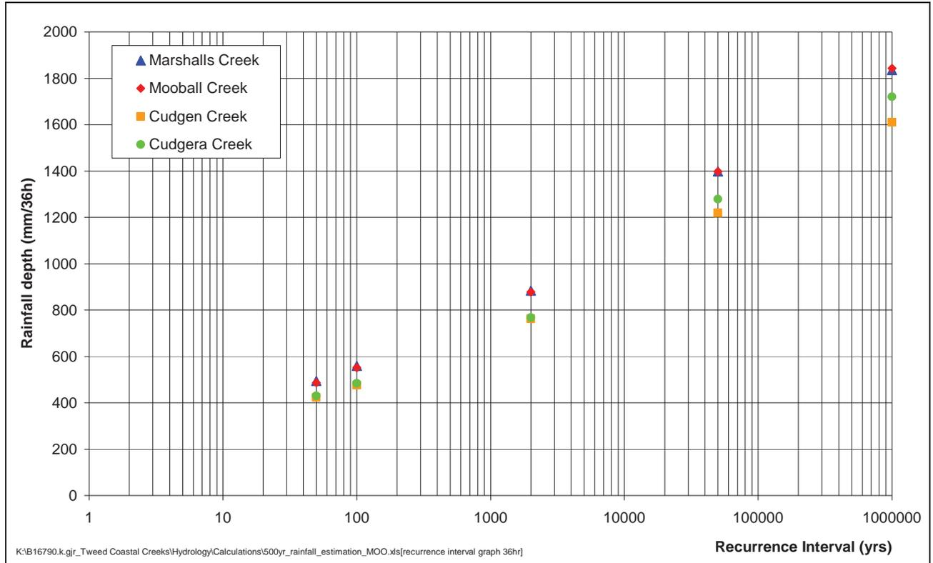
Figure 6-8 Design Rainfall Depths for a 36-hour Storm
