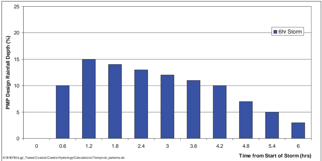
Figure 6-9 PMP Temporal Distribution – Short Duration Storm
