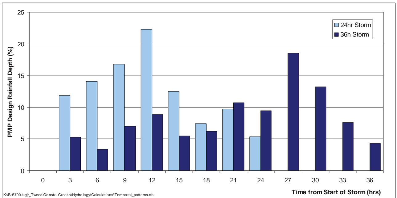
Figure 6-10 PMP Temporal Distribution – Long Duration Storm
