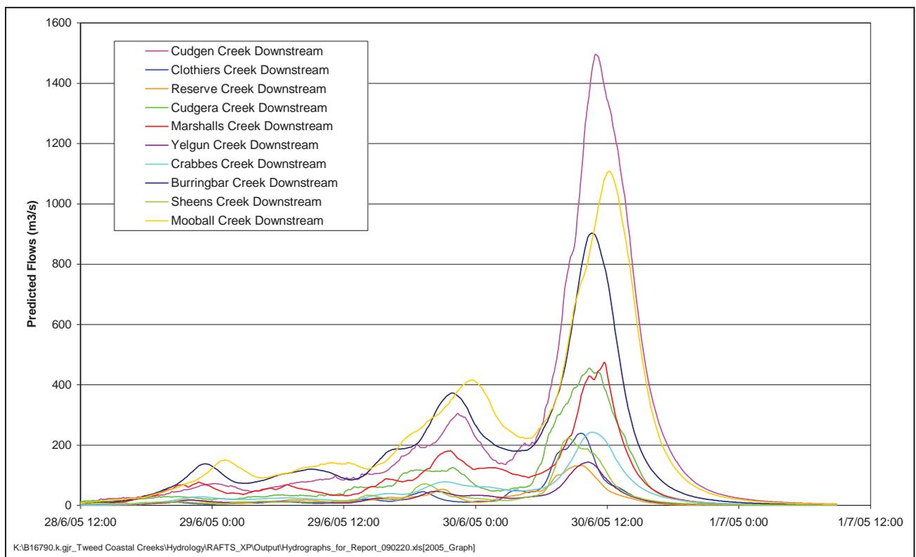
**Figure 5-7 RAFTS-XP Discharge Hydrographs – June 2005 Event**
