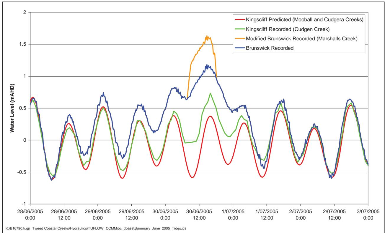
**Figure 5-8 Downstream Boundary Conditions – June 2005 Event**
