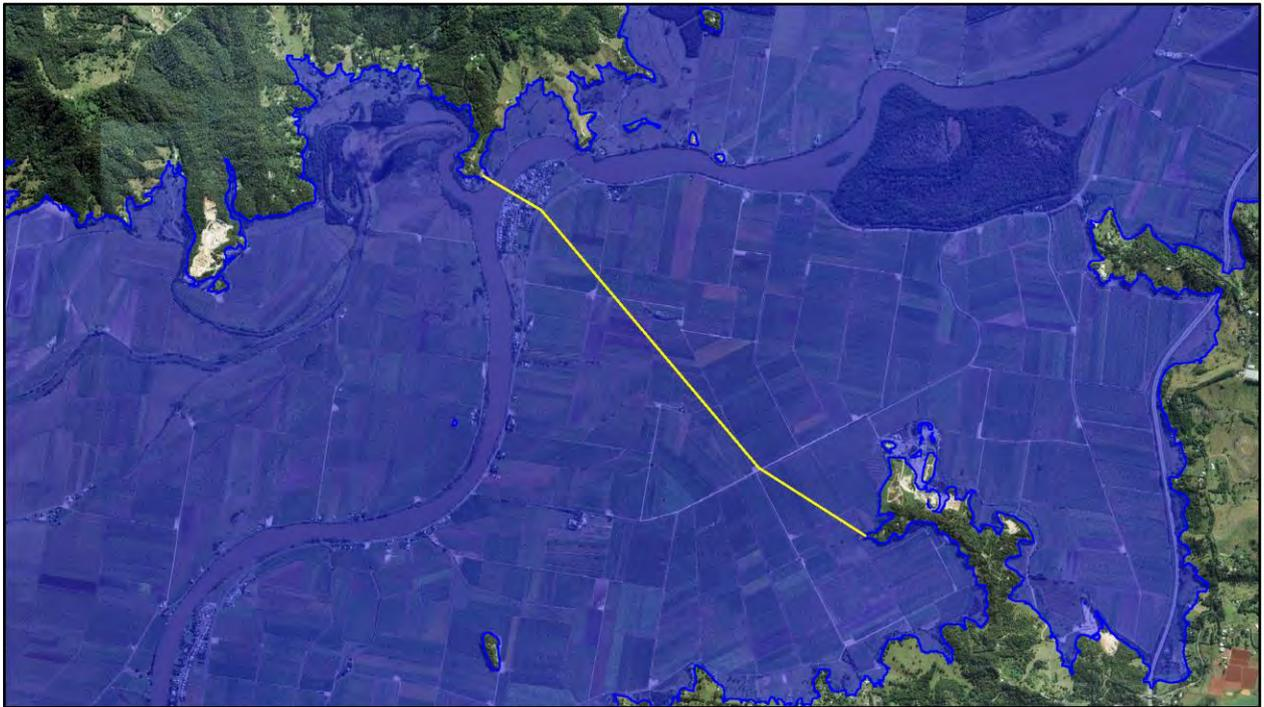
**Plate 10** Extent of cross-section (yellow) used to derive synthetic Tumbulghum rating curve for current study
