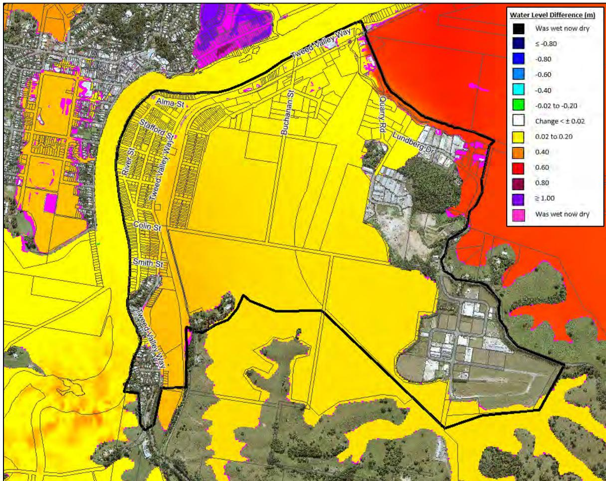
Plate 3 ARR2016 Flood Level Difference Map for 1% AEP flood
