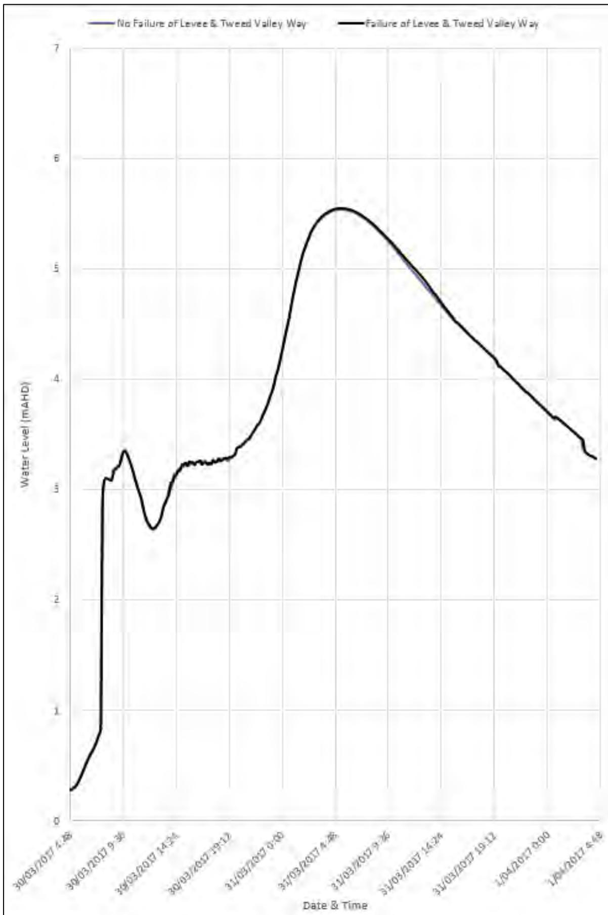
Plate C4 2017 Stage Hydrograph at Condong Creek flood gates
