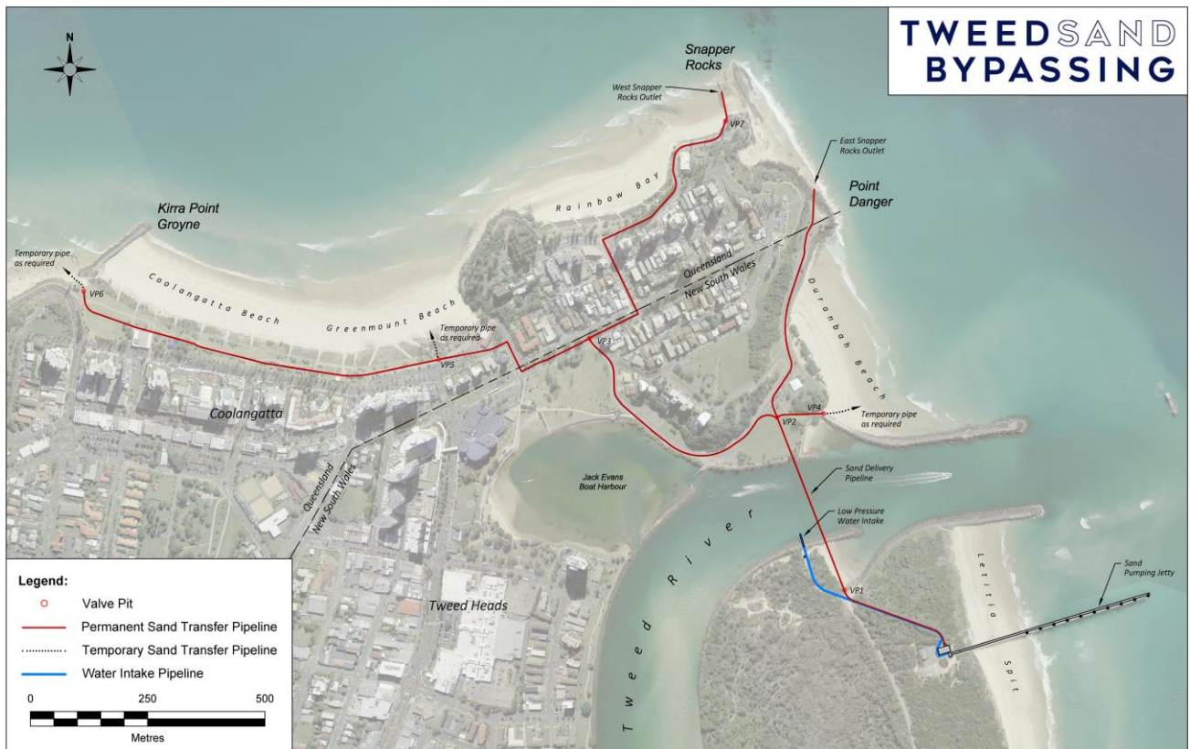
FIGURE 3-7 THE TWEED RIVER ENTRANCE SAND BYPASSING SYSTEM
