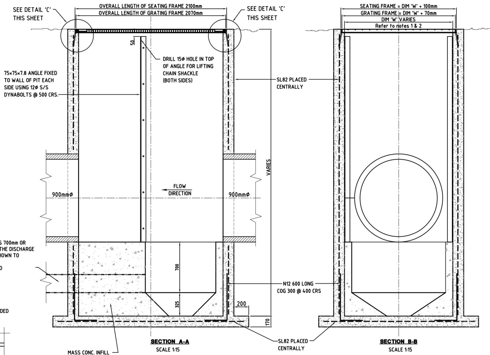
WHERE INVERT OF MAIN OUTLET PIPE IS 700mm OR GREATER ABOVE HIGH TIDE LEVEL AT THE DISCHARGE POINT, INSTALL 250 $\phi$  UPVC PIPE AS SHOWN TO PERMIT DRAINAGE/FLUSHING OF SUMP. OUTLET HEADWALL TO BE DESIGNED TO ACCOMMODATE THIS PIPE.
