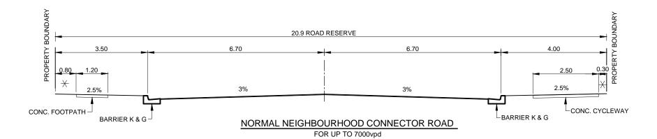
$\frac{\text{NOTE:}}{\text{TWEED SHIRE COUNCIL MAY CONSIDER STEEPER CROSSFALLS}} \\ \text{IN THIS ZONE WHERE TOPOGRAPHICAL CONSTRAINTS EXIST.} \\$
