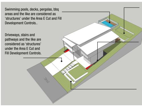
SEPP Exempt and Complying allows for 600mm retaining walls without consent. There is no limit on the number of these retaining walls allowing them to be tiered up a sloping site.
