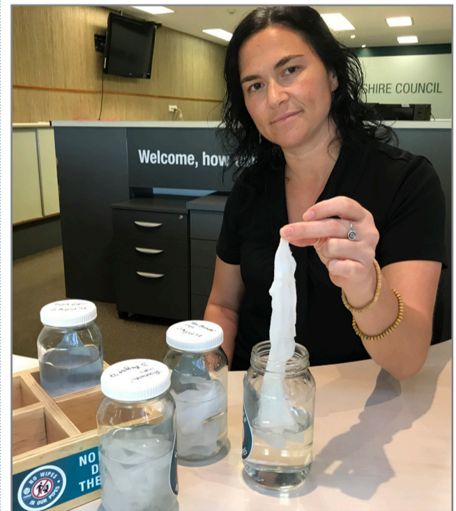
Customer Service Officer Rose Gomez finds that the wet wipe marketed as 'biodegradable' is still intact after 18 months in water. The one marketed as flushable is beginning to break down.
