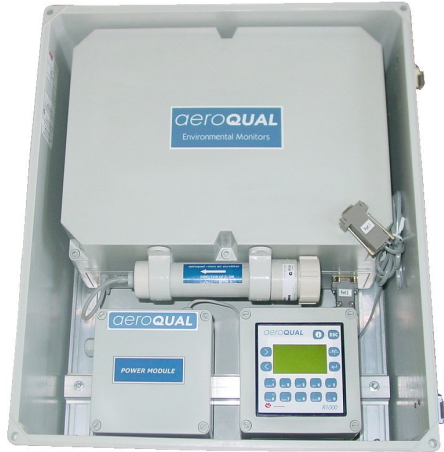
AQM 60 system installed in an external/outdoor enclosure and configured with multi-gas sensor module, zero-air scrubber, Programmable Logic Controller (PLC) and power supply module
