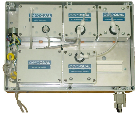
AQM 60 multi-gas sensor module with cover removed to show sampling pump, microcontroller module, four gas sensor modules plus temperature and humidity
